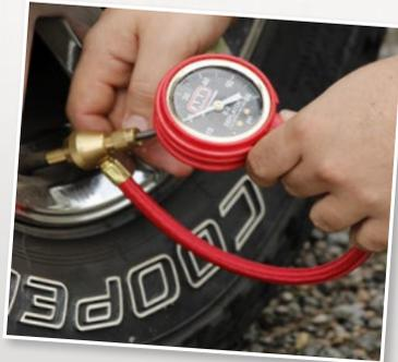
to build up which could lead to tyre failure. Low pressures increase rolling resistance, causing a reduction in fuel economy. You would also find a significant loss of steering precision and cornering stability. While an under inflation of 6psi doesn't seem like much, remember, it usually **represents about 20%** of the tyre's recommended pressure. You should also be aware that the load capacity of your tyres is reduced at lower pressures.
